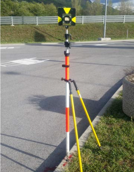
Figure 2. Tachymetric ground control point – reflector mount fixed onto concrete curb
