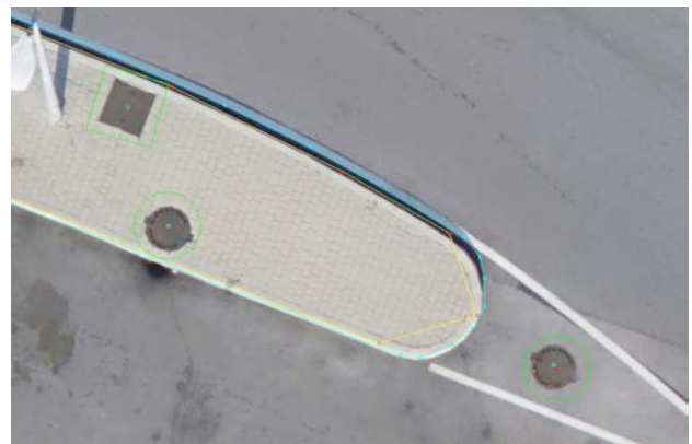
Figure 7. Part of a survey map – the above Figure 6 map with digital orthophoto overlay
