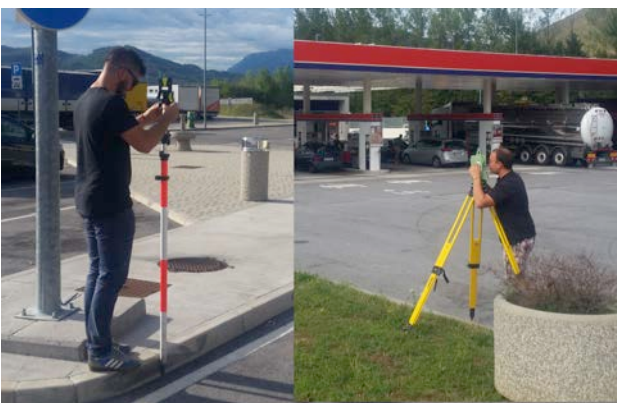
Figure 3. Validation survey with total station
